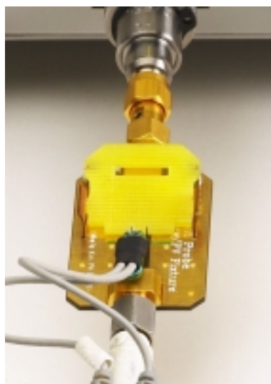
Fig. 2: Probe Deskew Fixture Allows Easy Connection of Probe Tip To 50-Ω Transmission Line
